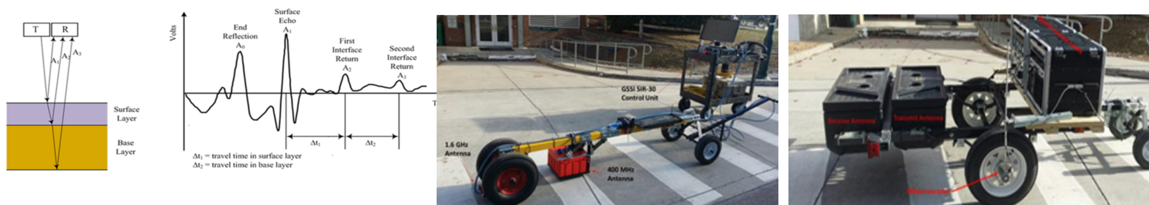
Figure 2. GPR operating principle and developed GPR systems
